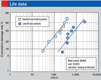
This chart shows the results of life testing under load conditions 50% of the basic dynamic load rating. The long life specification with special heat treatment shows L10 life 5 times or more that of the standard heat-treated products.
