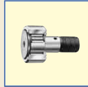
Cam Followers are bearings with a stud incorporating needle rollers in a thick walled outer ring. They are designed for outer ring rotation, and the outer rings run directly on mating track surfaces. Various types of Cam Followers are available. They are widely used as follower bearings for cam mechanisms and for linear motions.
