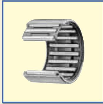
Shell Type Needle Roller Bearings are lightweight with the lowest sectional height among needle roller bearings with outer ring, because they employ a shell type outer ring made from a thin special-steel plate which is accurately drawn, carburized and quenched. Since these bearings are press-fitted into the housing, no axial positioning fixtures are required. They are ideal for use in mass-produced articles that require economy.
