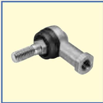
L-Balls are self-aligning rod-ends consisting of a special die-cast zinc alloy body and a studded ball which has its axis at right-angles to the body. They can perform tilting movement and rotation with low torque, and transmit power smoothly due to the uniform clearance between the sliding surfaces. They are used in link mechanisms in automobiles, construction machinery, farm and packaging machines, etc.
