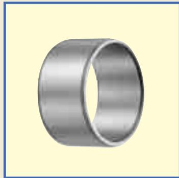
Inner Rings are heat-treated and finished by grinding to a high degree of accuracy and are used for Needle Roller Bearings. In the case of Needle Roller Bearings, normally the shafts are heat-treated and finished by grinding and used as raceway surfaces. However, when it is impossible to make shaft surfaces according to the specified surface hardness or surface roughness, Inner Rings are used.
