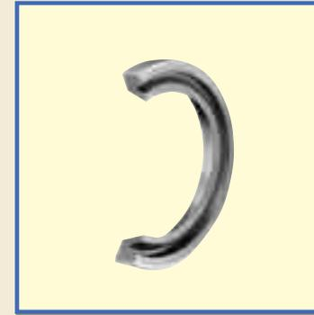
Seals for Needle Roller Bearings have a low sectional height and consist of a sheet metal ring and special synthetic rubber. As these seals are manufactured to the same sectional height as Needle Roller Bearings, grease leakage and the penetration of foreign particles can be effectively prevented by fitting them directly to the sides of combinable bearings.
