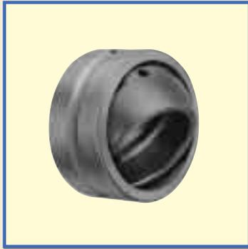
Spherical Bushings are self-aligning spherical plain bushings, which have inner and outer rings with spherical sliding surfaces. They can take a large radial load and a bi-directional axial load at the same time. They are divided into steel-on-steel types that are suitable for applications where there are alternate loads or shock loads, and maintenance-free types which require no lubrication.
