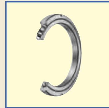
Crossed Roller Bearings are high-rigidity and compact bearings with their cylindrical rollers alternately crossed at right angles to each other between inner and outer rings. A single Crossed Roller Bearing can take loads from any directions at the same time such as radial, thrust, and moment loads. These bearings are widely used in the rotating parts of industrial robots, machine tools, medical equipment, etc. which require compactness, high rigidity and high rotational accuracy.
