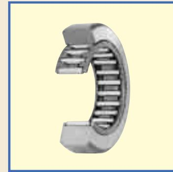
Roller Followers are bearings in which needle rollers are incorporated in a thick walled outer ring. These bearings are designed for outer ring rotation, and the outer rings run directly on mating track surfaces. They are used as follower bearings for cam mechanisms and for linear motions.
