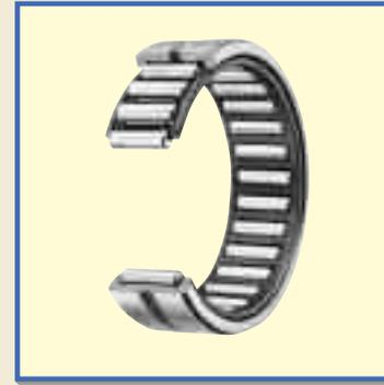
Machined Type Needle Roller Bearings have an outer ring made by machining, heat treatment, and grinding. The outer ring has stable high rigidity and can be easily used even for light alloy housings. These bearings are available in various types and optimally selectable for different conditions such as heavy loads, high-speed rotation and low-speed rotation. They are most suitable for general-purpose applications.
