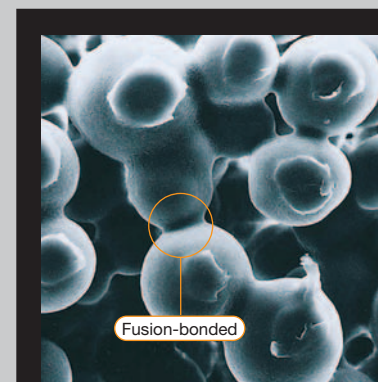
Before impregnating oil Resin particles are strongly fusion bonded.
